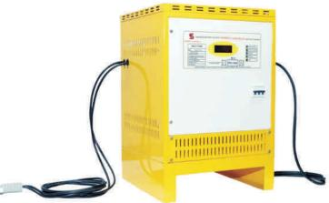
TC Series battery chargers are comes with taper current (DIN41772) profile. Due to taper current profile battery life will be enhancing moderately. These chargers are used to charge C5 rating traction batteries like flooded batteries, VRLA batteries & Gel batteries of 12V, 24V, 30V, 36V, 48V, 72V, 80V & 110V and Current starts from 5 amps to 200 Amps
